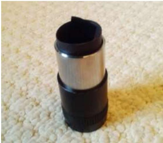
Once the roll has been stuck together, remove the card from the eyepiece. Trim off any protruding tape, or fold it over and stick it down. Secure the outside of the roll with a piece of tape in a similar manner.
