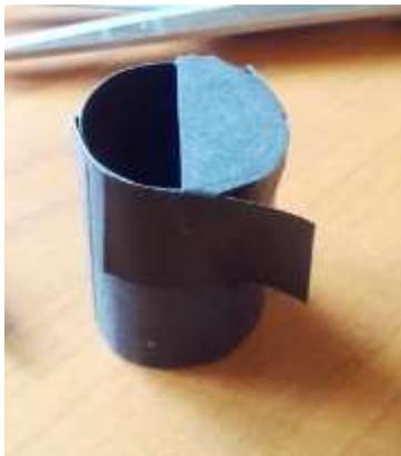
When you are happy that all is secure, check for any small holes and make sure that these are masked with more small pieces of tape. This is to ensure that light does not come through the shielded part of the occulting bar.
