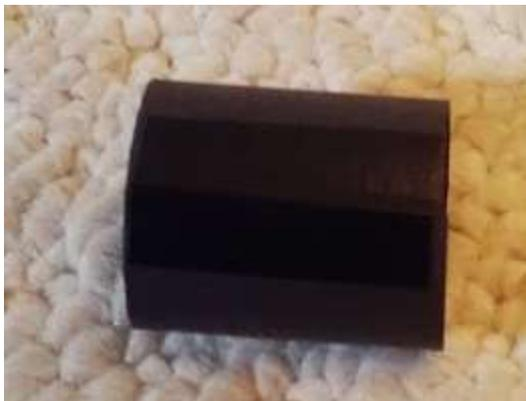
Once you are happy the roll of card is properly secure, place it back into the eyepiece barrel and slide it backwards and forwards to see how well it fits.
