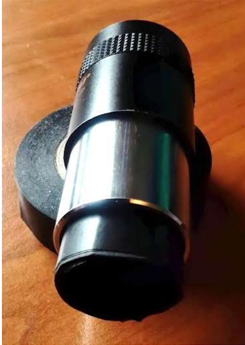
When the eyepiece is placed in the focuser of the telescope, the occulting bar will now obscure light coming into your eye from one side of the telescope.
